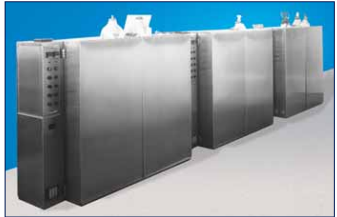
THREE CUSTOM MADE CYLINDER WARMING OVENS EACH DESIGNED TO OPERATE IN A ZONE 2 HAZARDOUS AREA & CERTIFIED TO EU ATEX DIRECTIVE 94/9/EC. EACH CHAMBER ACCEPTS FIVE 1620x255mm CYLINDERS
