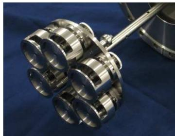
The target manipulator accommodates up to six 1-inch diameter targets. The selection of the target is done through a controlling computer. Each of the individual targets rotates about its axis, providing a uniform erosion of the target when using with a laser scanning system.
