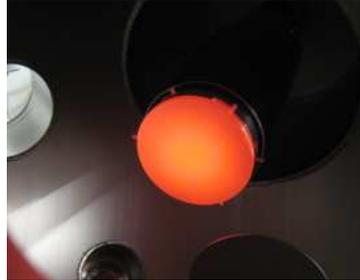
The deposition stage welcomes substrates up to 2-inch. It has a high temperature oxygen resistant heater in order to enhance crystalline structure for simple element coatings and complex ceramic compound. The deposition stage is supplied with a motorized rotation and X-axis for improving uniformity of the films.
